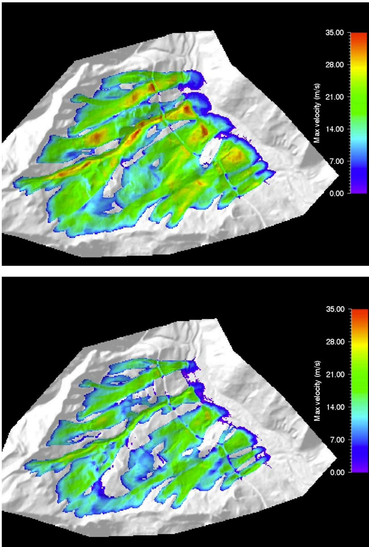
Figure 6. Simulated maximum velocities of the extreme scenario (300y top), the intermediate scenario (100y middle) and the frequent scenario (10y bottom)
